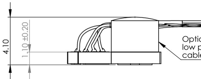
Optional thermometer or low power heater below cable entry
