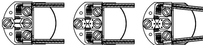
When very short samples are used, the WP100 must be mounted at an angle and the sample contacts will be slightly further from the sample.
