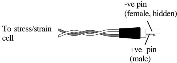
**Figure 1. A LEMO FGG.0S.302.ZLAT connector indicating polarity. Note that as this is a hermaphrodite connector, the one on the cryostat cable will have the opposite polarity.**
