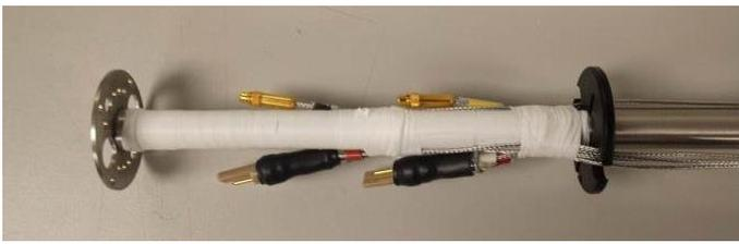
7. Connect the cables to the new top plate. The coax with the yellow band should be connected to the SMA connector marked “High”, the one with the black band to the one marked “Low”. The drive cables connect so that the coloured bands match the wires they are connecting too. In case the feed throughs have been removed from the plate, compression is blue/brown and tension is red/white.
