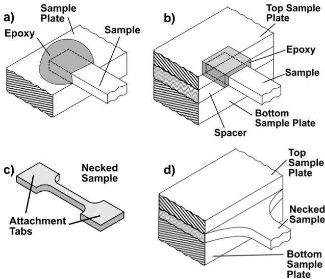
**Figure 2.** a) It is possible to simply glue the sample to sample plates with a drop of epoxy. b) A better mounting method achieves higher strain homogeneity. c) A necked sample. d) A Necked sample mounted between sample plates.
