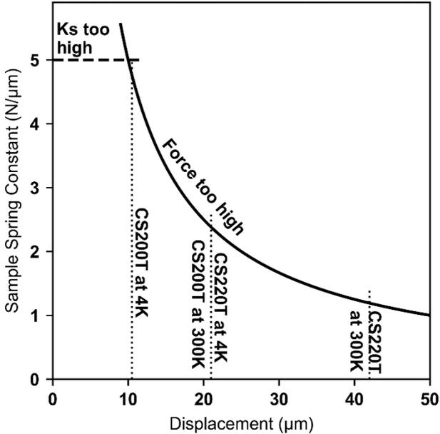
Figure 1. Recommended operating envelope for CS2x0 series cells. Sample spring constant ( $K_s$ ) should be limited to about 5 N/μm, and force to about 50 N to avoid unwanted twisting of the cell. In other words, the sample spring constant and displacement should be chosen to lie below the solid line. Maximum displacements of the cells are marked for convenience. There is no problem using either cell at e.g. 9 μm and 4.5 N/μm.
