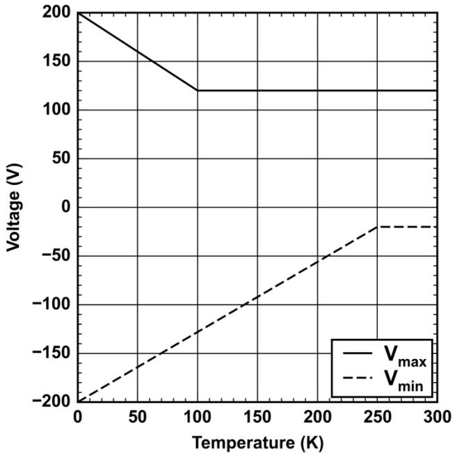
Figure 4. Recommended voltage limits for various temperatures.
