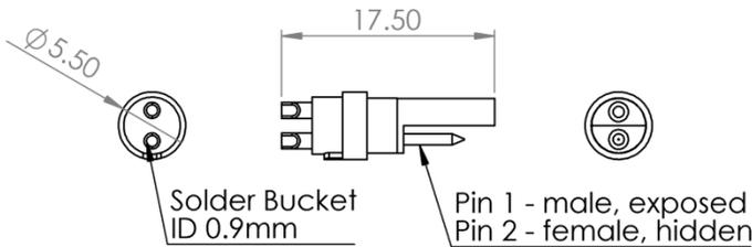
**Figure 3. Lemo FGG.0S.302.ZLAT connector. This connector is hermaphroditic, i.e. it mates with another copy of itself. Pin 1 mates with pin 2 and vice versa.**
