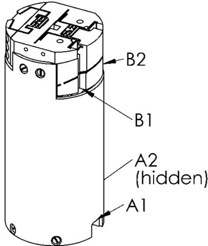
**Figure 2. Wire exit points. A1 and A2 are openings on the bottom edge of the cells 180° apart. They are large enough for all the wires, which can exit vertically or horizontally. B1 and B2 are small slots allowing wires to exit upwards. Max 4 wires per slot. The default configuration is drive wires through A1 and capacitance cables through A2.**
